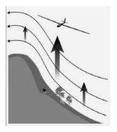
When the wind blows at the face of a long hill or ridge, it is deflected upwards. If we fly a glider in front of the hill, it will be pushed upwards too. Depending on the wind strength the lift may extend to two or three times the height of the hill. Unless well above the hilltop, we always stay in front of the hill, making all turns away from it, because the air descends behind the crest of the ridge. This is known as curlover or a "clutching hand".
