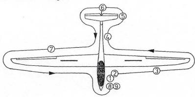
While walking around the glider, check the surface for cracks, bucklings or unevenness or any unusual feature. In case of doubt call an expert for a professional opinion.
