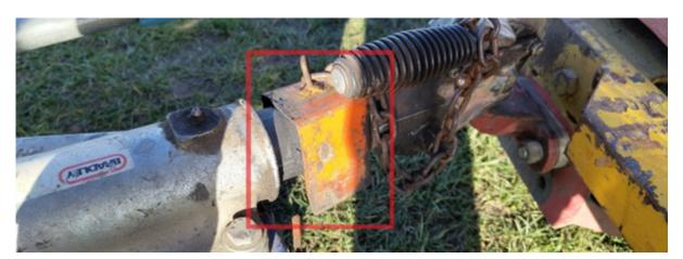
**4** — This is used to allow you to reverse the winch. It must be in place whilst reversing or the winch's wheel brakes will activate. Remember to remove this before moving off!
