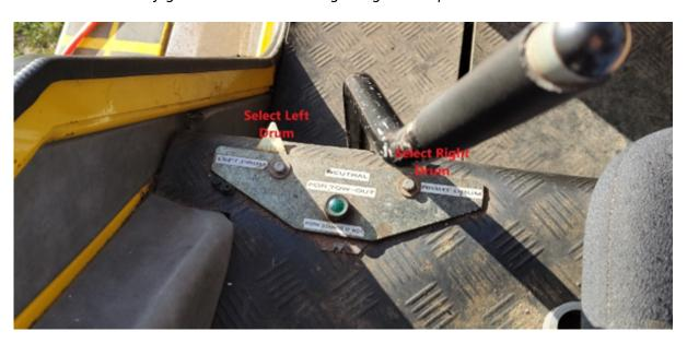
The handle on the left-hand side of the winch's cabin is used to switch between the left drum, neutral (middle) and right drum.
