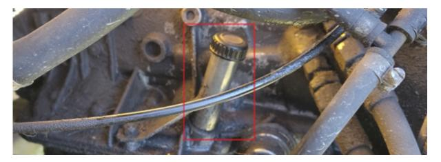
**3. Transmission Fluid Dipstick** — There is a small screw-on dipstick here which can be used to check the transmission fluid levels.
