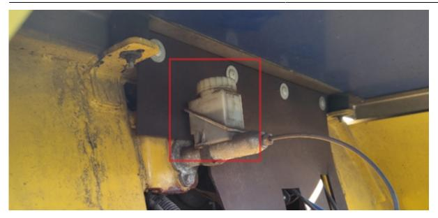
Finally, this is the brake fluid reservoir. Ensure there is brake fluid in it!
