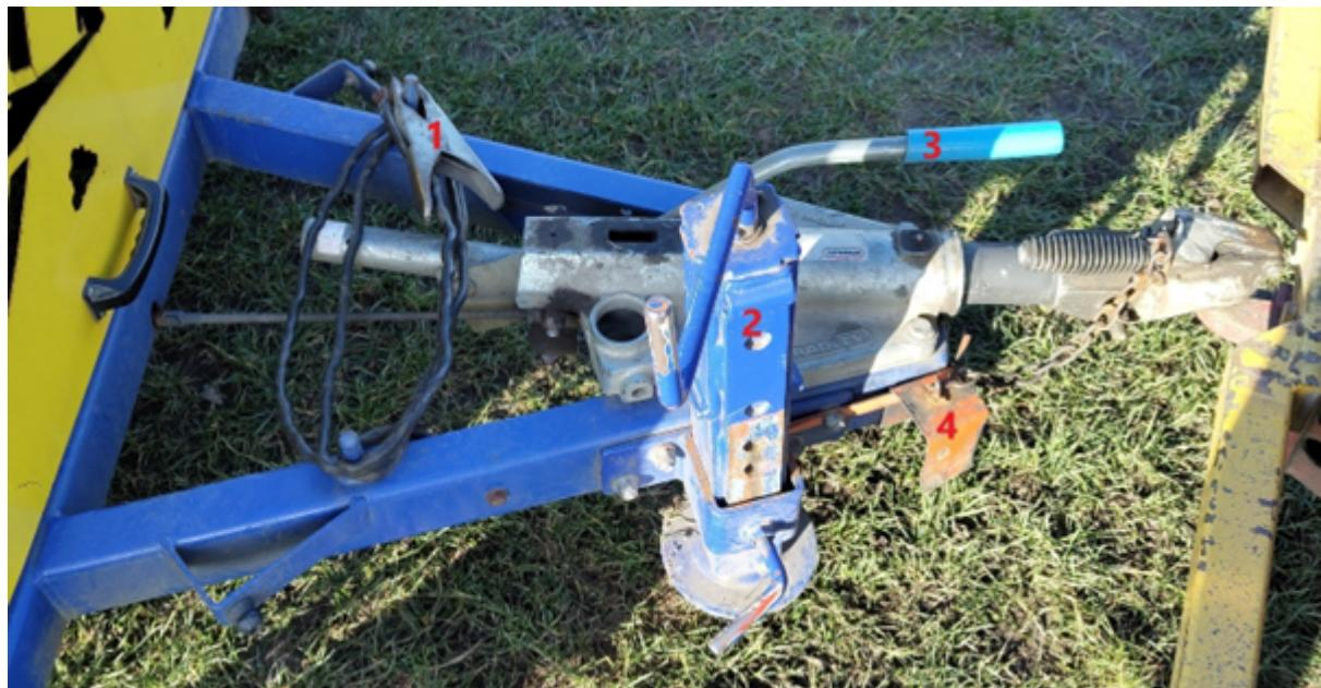
**1. Earthing Clamp** — This should be attached to the earthing stake. See above.
