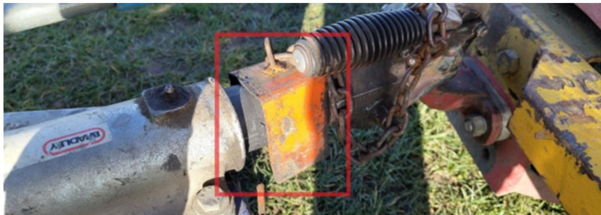
**4** — This is used to allow you to reverse the winch. It must be in place whilst reversing or the winch's wheel brakes will activate. Remember to remove this before moving off!
