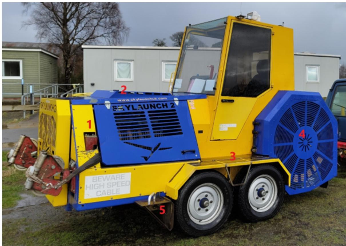
**1. Guillotine** — Each cable has its own guillotine. It is a relatively sharp piece of metal attached to a large spring which is held under compression. The guillotine is only used when the glider is unable to release the cable and is activated by the winch driver using the large red handle in the cabin. Operating the handle cuts both cables at the same time.
