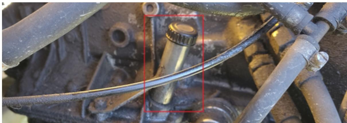
**3. Transmission Fluid Dipstick** — There is a small screw-on dipstick here which can be used to check the transmission fluid levels.
