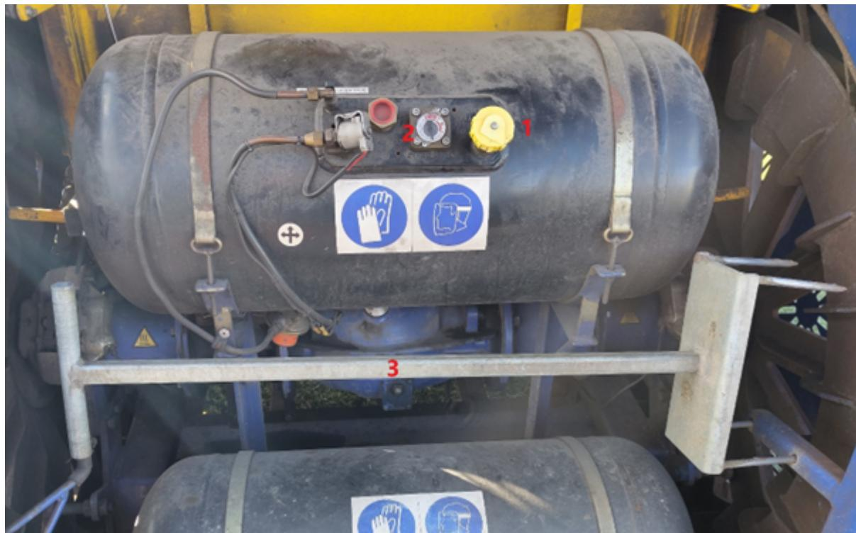
**1. Fuel Cap** — This cap covers the LPG tank's valve. It should be kept on apart from when refuelling the winch.
