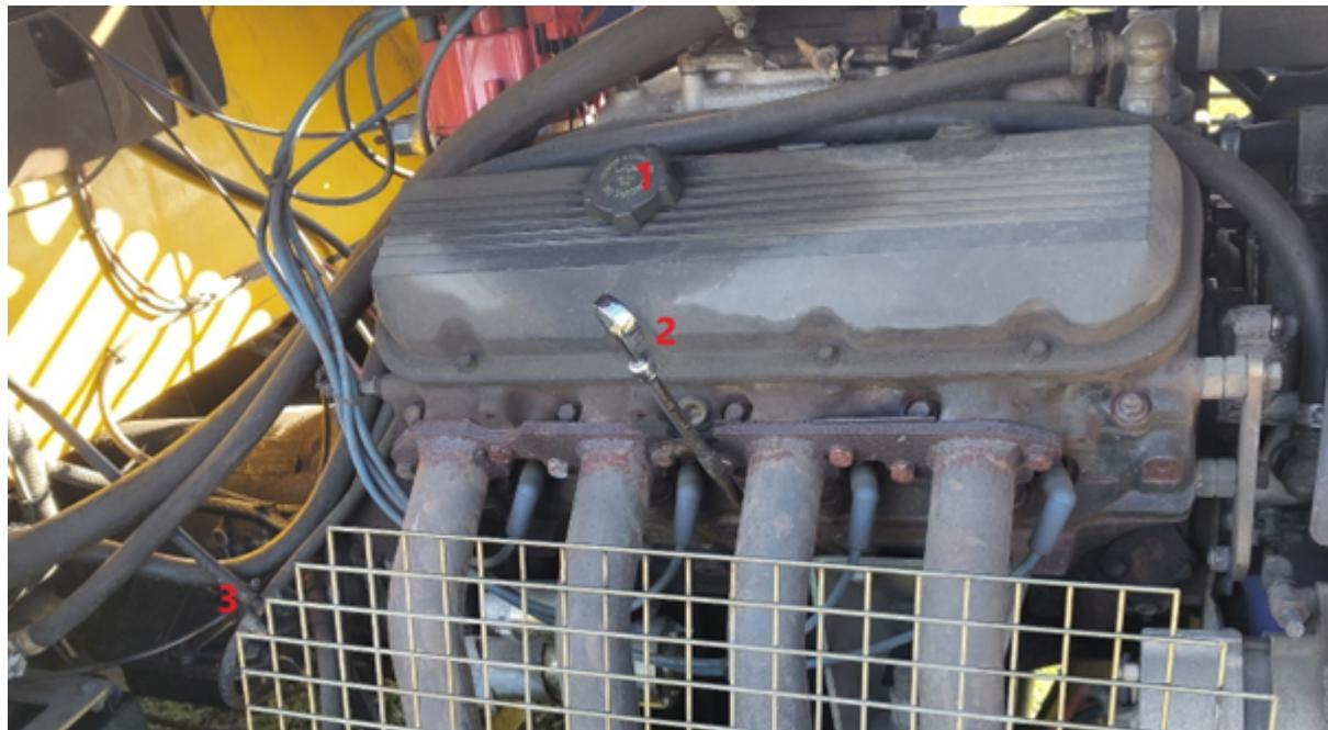
**1. Oil Filler Cap** — Use this to top-up the winch's oil.
