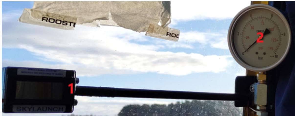
**1. Launch Assist** — Some gliders are fitted with a Launch Assist transmitter which broadcasts the aircraft's indicated airspeed (IAS) during a winch launch. This display is connected to a receiver, but it can be up to 2 seconds out-of-sync. Launch Assist should not be solely relied upon and is only an additional aid – it can, however, be very helpful when launching an early student who may struggle to stay stable during the launch.
