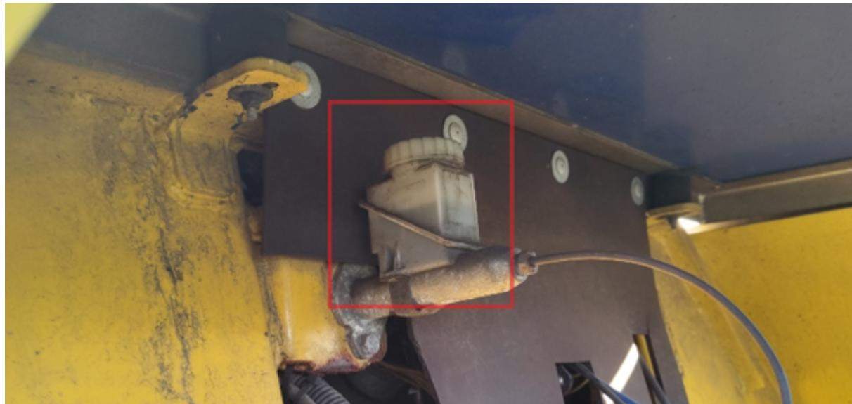
Finally, this is the brake fluid reservoir. Ensure there is brake fluid in it!
