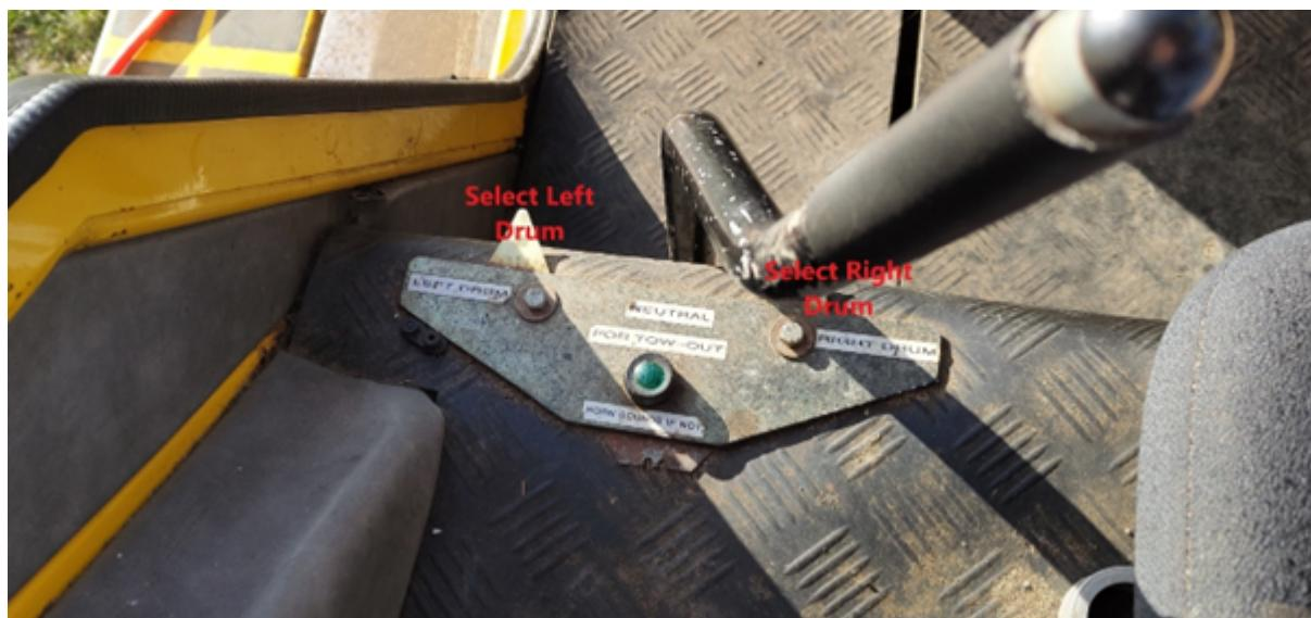
The handle on the left-hand side of the winch's cabin is used to switch between the left drum, neutral (middle) and right drum.
