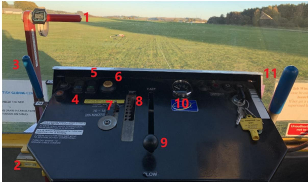
**1. Guillotine** — When the guillotine lever is pulled, two large and heavy compressed springs ram a sharp piece of metal into the cables, cutting them. The guillotine should only be used when the glider is unable to release, which is very rare.
