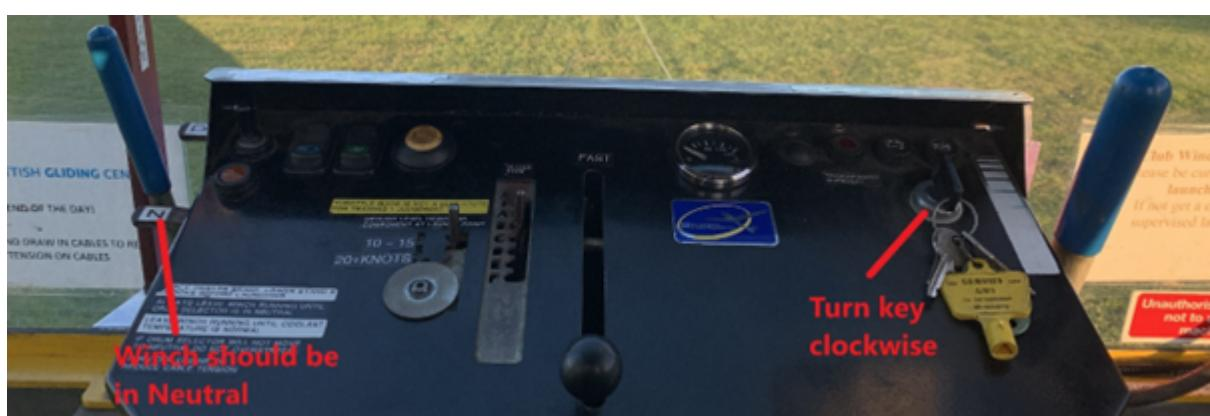
Ensure that the winch is in Neutral, and the drum selector is in the middle. Then, whilst applying some above-idle power (this is only required when the winch is cold), turn the ignition. It may take several seconds for the winch to start whilst it is cold. Leave the winch running to allow it to heat up whilst you take the first set of cables down to the launch point.
