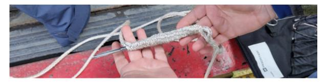
Once all the cable has been fed through the inside of the other end, remove the fid. The cable's end should still be attached to the fid.
