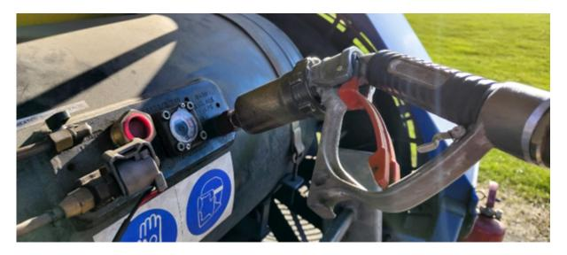
Remove the yellow cap from whichever tank you wish to fill. Carefully screw on the hose to the tank's fitting. Be careful not to under- or over-tighten the connector. Open the hose's valve and use the clip to hold it open – there may be some leakage of LPG when you do this.
