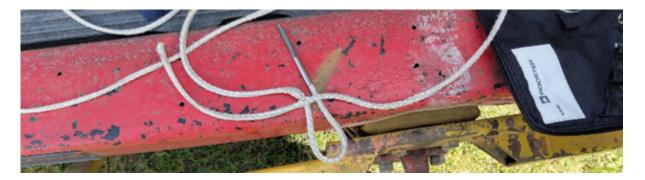
Working away from the cable's broken end, push the fid through the cable 3 times.
