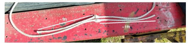
Mark each end of the cable, leaving around a foot of extra cable on each end.
