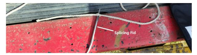
Attach either end of the cable to the splicing fid (which can be found in the blue wallet in the winch's cabin). Then, push the splicing fid (with the cable end attached) through the mark you placed on the other cable end.
