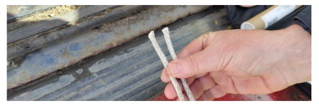
Trim the cable using a pair of scissors to remove the frayed ends.
