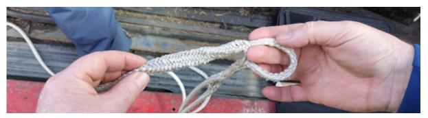
After the 3rd time, push the fid into the cable (instead of pushing all the way through). Carefully feed the fid through the centre of the cable.
