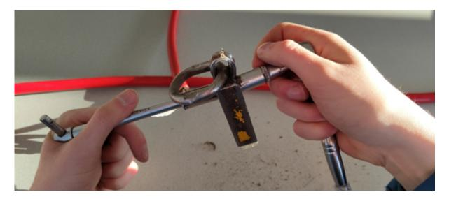
Then, place the strop's shackle over the weak link assembly, and insert and tighten a nut and bolt. Again, it should be relatively tight whilst allowing some movement with resistance.
