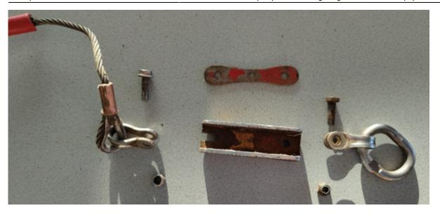
Using a ratchet, remove the bolt from the weak link assembly and the strop.
