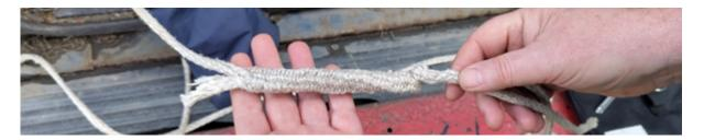
Detach the cable end from the fid, then using a pair of scissors, further trim the cable end to create a smaller point.
