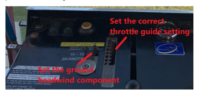
Check the throttle guide setting sheet for the appropriate launch characteristics of the glider you are launching. Set the appropriate surface wind component and throttle guide setting.
