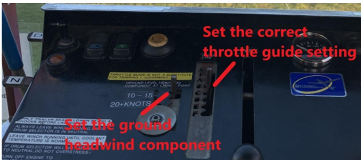
Check the throttle guide setting sheet for the appropriate launch characteristics of the glider you are launching. Set the appropriate surface wind component and throttle guide setting.
