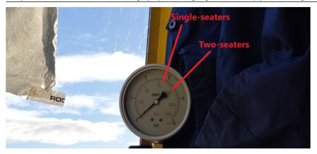
The pressure gauge shows the amount of pressure that the cables are placing on the winch's transmission. It can be a good indicator of how well a glider is being launched.
