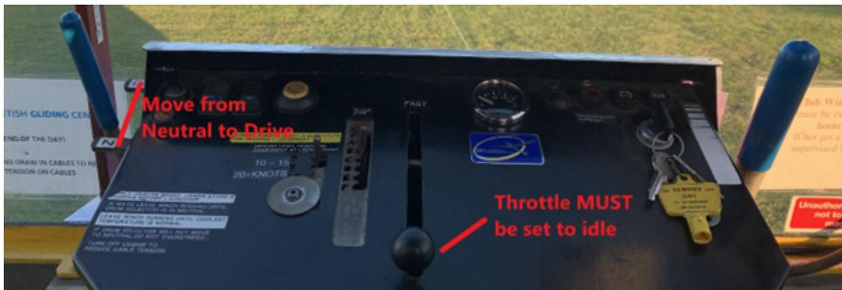
Once you have confirmed that the take up slack light signal is slowly flashing, put the winch into Drive. **You should now be fully focused on the light.**
