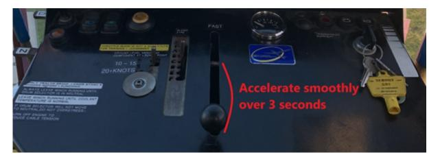
Over a period of around 3 seconds, steadily increase power to the required level. This often may be the throttle guide, but the glider may require more or less power depending on the conditions. **Remember: the throttle guide is a <u>guide</u>**, not an absolute solution. You can always push through the guide if you need more power.
