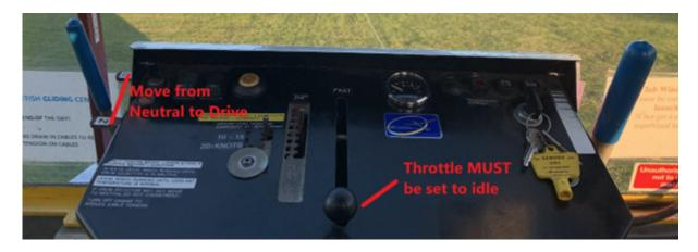
Once you have confirmed that the take up slack light signal is slowly flashing, put the winch into Drive. **You should now be fully focused on the light.**
