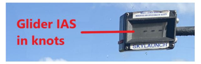
The winch is fitted with a Launch Assist receiver. The club gliders, and a few private ones, are fitted with a special transmitter which broadcasts the glider's indicated airspeed (IAS) during a winch launch. Keep in mind that **you should not try to chase the speedometer** and it can be up to 2 seconds out-of-sync.
