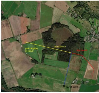
the height of the glider in circuit or its line in the circuit, the launch may be stopped earlier or later. Deciding on this point comes with experience and if in doubt use the line shown in the diagram. Get help from an instructor or qualified pilot with this decision making.
