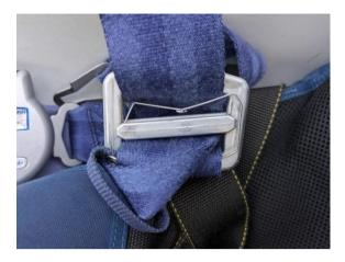
We had an incident recently where the strap in the Perkoz was loose during aerobatics. Luckily, the pilot managed to recover from this without incident. The spring clip was bent and in the wrong position. It could not be put into the correct position. With these types of straps it can happen that the spring gets bent when the strap is twisted and then it can become loose. Check the straps and report any problems.
