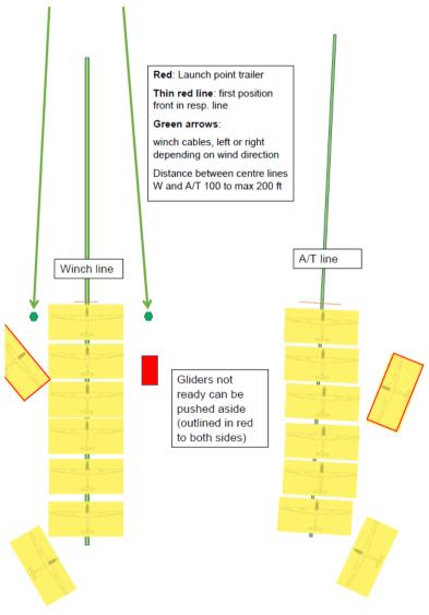
To avoid delays at the launch point when both cables are out, always have the 1<sup>st</sup> glider in position far enough in front of the caravan so that the 2<sup>nd</sup> glider also has its wingtip in front. Make sure that pilots in both gliders are ready to launch. As soon as they are launched, the next 2 gliders are moved forward while the cables are retrieved.
