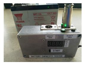
Once connected to the Capacity Check connector the display will show battery voltage.
