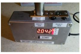
Volts (V) values. When the Capacity Check is complete it will display only the Ah capacity of the battery.
