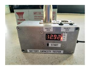
Pressing the START button will commence a test cycle. During the cycle the display will rotate through Ampere hours (Ah), Amps (A) and
