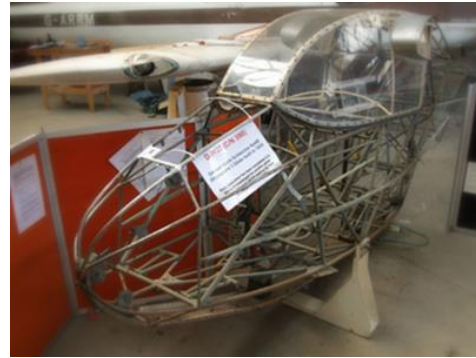
Fabric covered tubular steel fuselage
