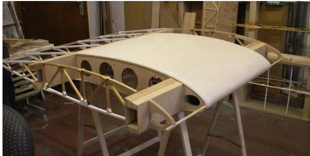
Plywood covered D box
