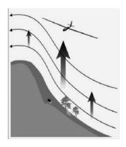
When the wind blows at the face of a long hill or ridge, it is deflected upwards. If we fly a glider in front of the hill, it will be pushed upwards too. Depending on the wind strength the lift may extend to two or three times the height of the hill. Unless well above the hilltop, we always stay in front of the hill, making all turns away from it, because the air descends behind the crest of the ridge. This is known as curl-over or a "clutching hand".
