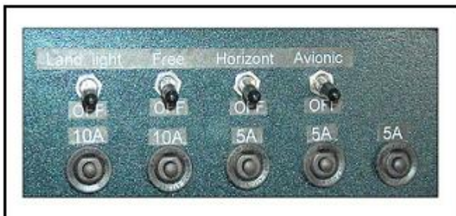
Example of switch and fuse layout
